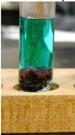
Solid copper metal is produced. It is brownish orange, just like a penny. It is forming on the outside of the zinc metal at the bottom of the test tube. As the amount of solid copper that is formed increases, the amount of copper metal ions that are dissolved in the solution decreases. Eventually, the solution will become less blue, because the blue color of the solution is due to the presence of dissolved copper. The solid zinc metal, on the other hand, disappears as it dissolves.
