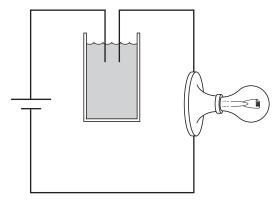
The above picture shows a light bulb connected to a battery with the circuit interrupted by a solution. When dissolved in the water to form a 1.0 molar solution, all of the following substances will complete a circuit allowing the bulb to light *except*
